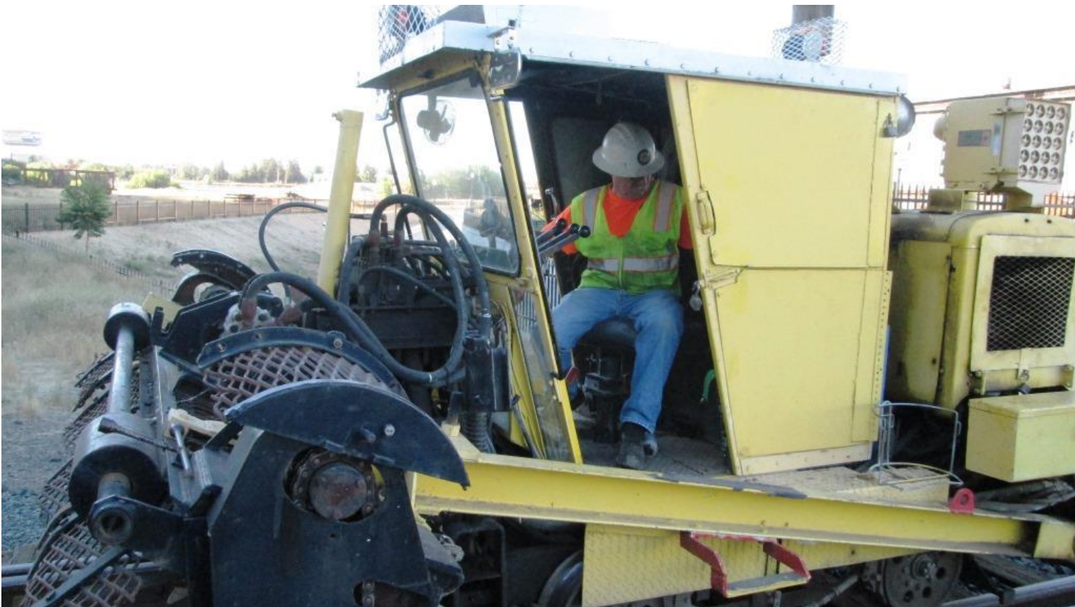
Mike H. tests the scarifier with its new compressor on the 560 Track
