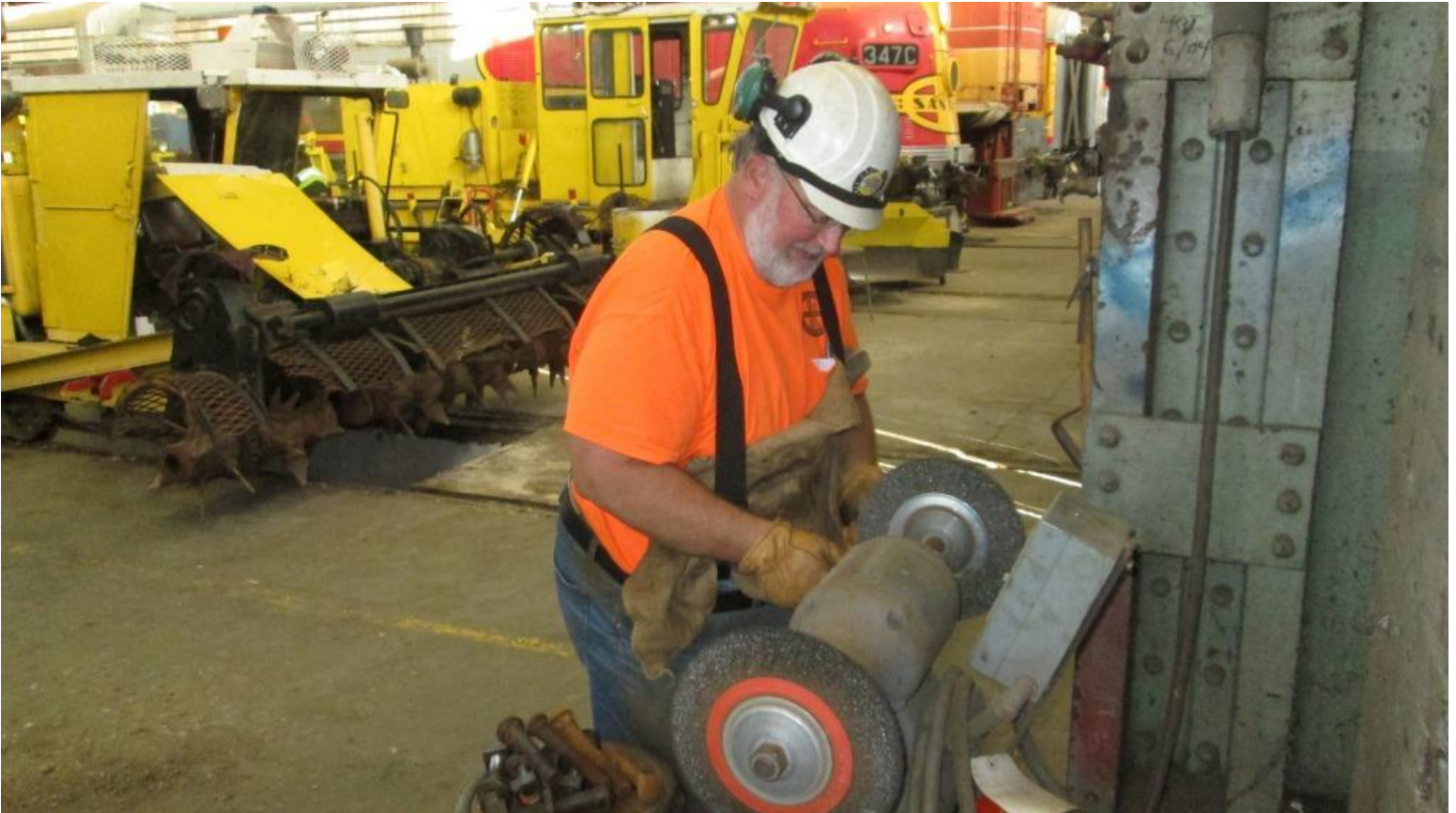
Frank uses the wire-brush to clean bolts
